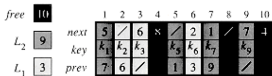
Figure 11.8 Two linked lists, L_1 (lightly shaded) and L_2 (heavily shaded), and a free list (darkened) intertwined.
